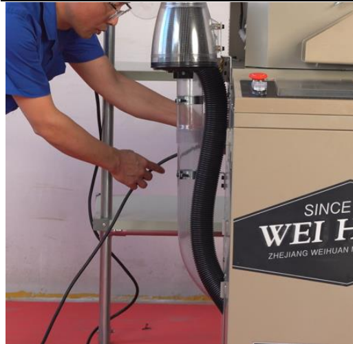
将感应线插入机箱 put the cable to controller box
