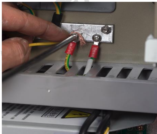
黄绿线和机箱地线连接，黑色感应线连接长电线 green+yellow cable connect to machine ground wire, extension the length of black cable with others wire
