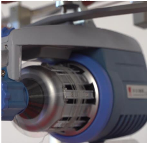
将储纬器的灰色报警线与线架连接 the grey cable of device connect to creel
