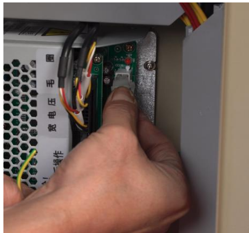
打开机箱，白色插头和控制盒右侧白色插孔连接 open the controller box, join two white connector(KDF) together in right side of controller box
