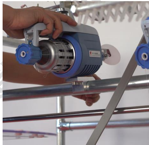
线架加装一根钢管，储纬器一个装在中间，一个装在右侧 add a horizon pipe for creel, put one of IRO device on middle of creel and another is on right side
